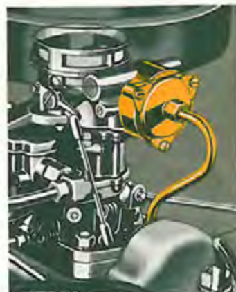
Modern Packard design specifies automatic choke to shorten warm-up and save gasoline.
