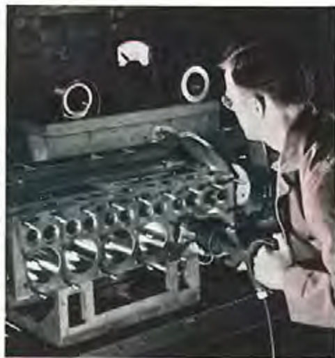
Harnessing the accuracy of electricity is another development for fine measurement. It is used here in checking diameter of cylinders.
