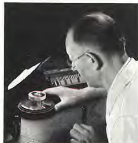
The Supreme Court of all measurement is this superaccurate light ray machine which checks gauges to a tiny millionth of an inch.
