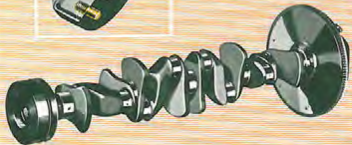
Packard crankshafts are heavy forgings with integral counterweights. They are 100% balanced and main and crankpin bearings overlap, serving to further stiffen the shafts and smooth out engine vibration.
