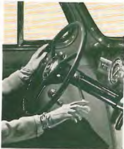
Handishift puts the gear change lever on the steering column, closer to hand for quicker operation. Shifting is easier.
